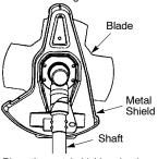
Place the metal shield under the gearbox, and align the screw holes.
